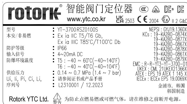
Fig. L-6: YT-3700 Intrinsic safety type (CCC)
