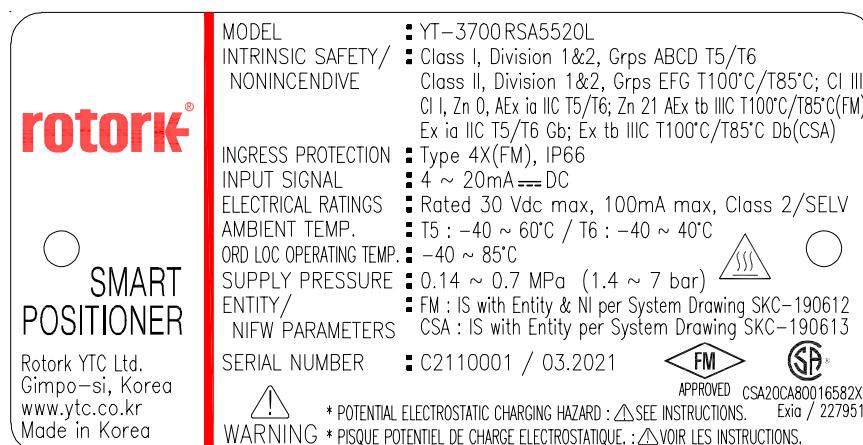
Fig. L-4: YT-3700 Intrinsic safety type (FM, CSA)
