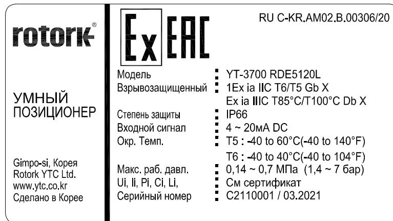
Fig. L-5: YT-3700 Intrinsic safety type (EAC)
