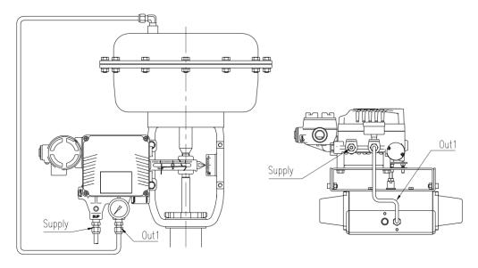
Fig. 5-1: Single acting linear actuator
