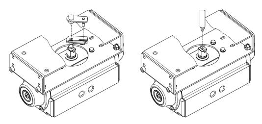
Fig. 4-17: Main shaft center alignment (Fork lever) Fig. 4-18: Main shaft center alignment (Namur)
