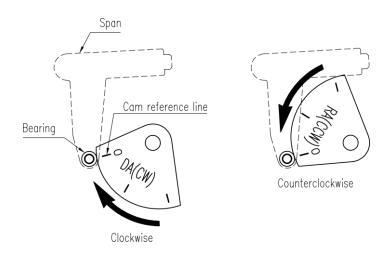
Fig. 7-4: Cam Installment (Da)
