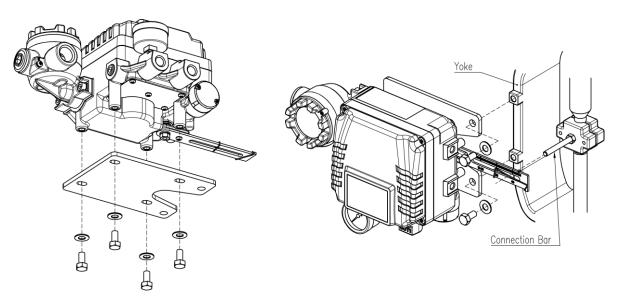
Fig. 4-3: Attaching positioner to bracket
