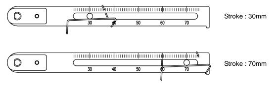
Fig. 4-8: Feedback lever and location of the connection bar
