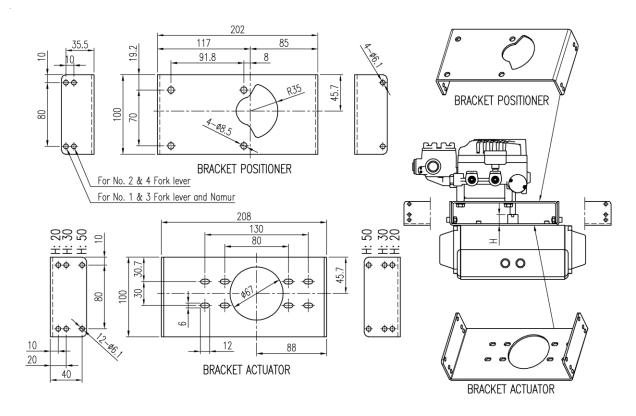
Fig. 4-12: Brackets and positioner
