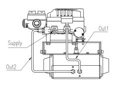
Fig. 5-6: Double acting linear actuator
