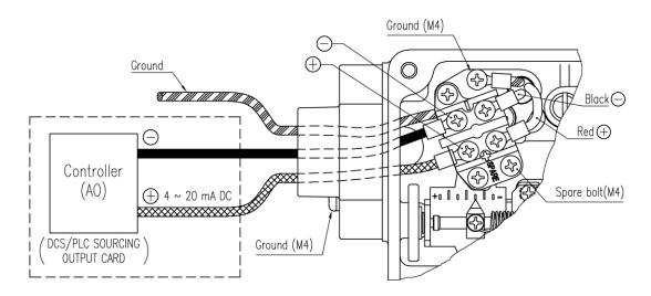
Fig. 6-4: Connecting cables
