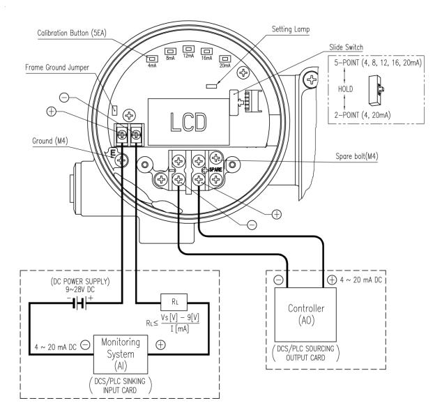
Fig. 6-6: Connecting cables
