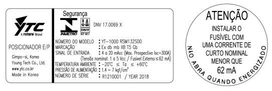
Fig. L-13: YT-1000 Ex db mb IIB T5 Gb (INMETRO)
