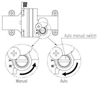
Fig. 7-13: A/M switch adjustment
