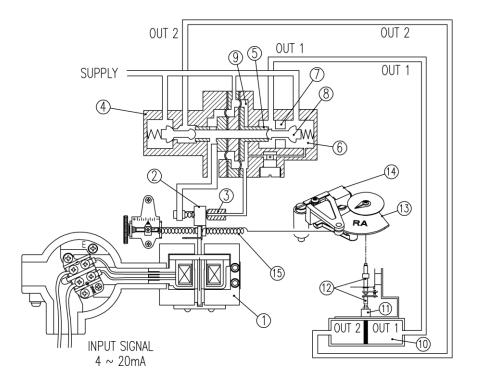
Fig. 3-2: Rotary positioner with an actuator
