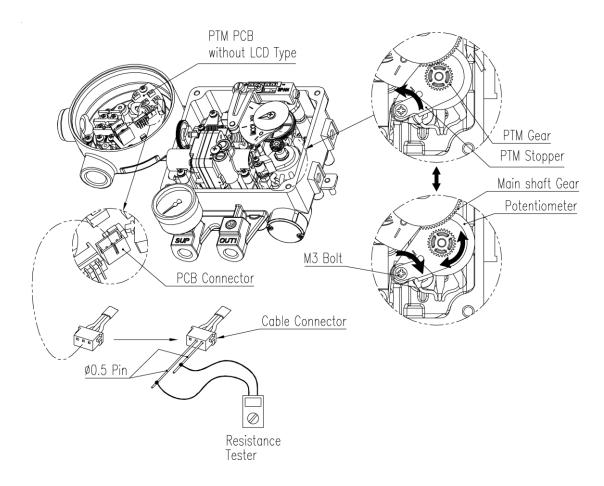
Fig. 7-15: Resetting resistance of potentiometer (without LCD)
