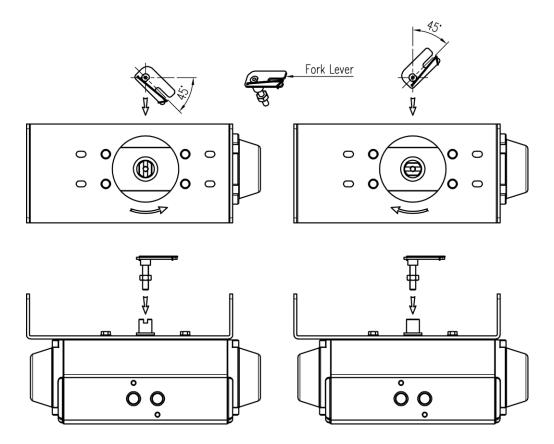
Fig. 4-15: Counter-clockwise and clockwise rotation.
