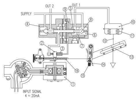
Fig. 3-1: Linear positioner with an actuator
