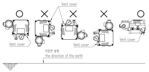
Fig. 4-1: The correct positions of a vent cover
