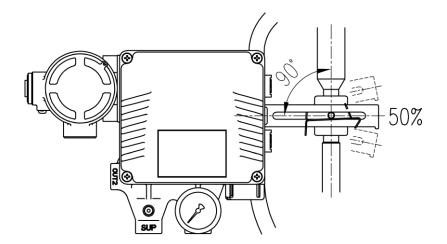
Fig. 4-7: Feedback lever and valve stem
