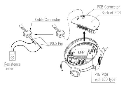
Fig. 7-16: Resetting resistance of potentiometer (with LCD)
