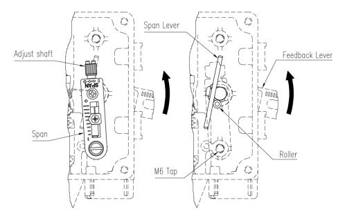
Fig. 7-3: Span Installation (Ra)
