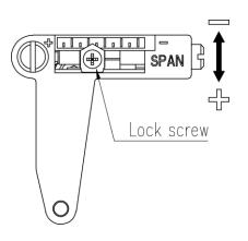
Fig. 7-10: Rotary span unit
