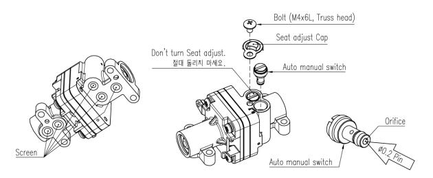
Fig. 8-1: Pilot unit and Auto manual switch
