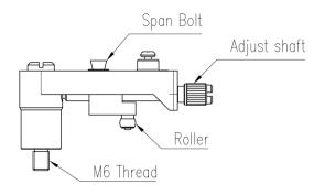
Fig. 7-2: Linear span assembly
