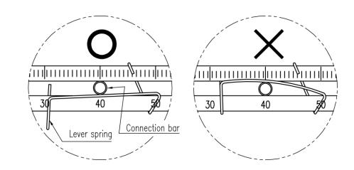
Fig. 4-6: Proper way to insert connection bar between feedback lever and lever spring
